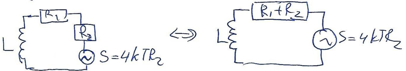
$$k(\omega) = \frac{i\omega L}{i\omega L + R_1 + R_2}; \quad S_L(\omega) = \left| \frac{i\omega L}{i\omega L + R_1 + R_2} \right|^2 \underbrace{4kTR_2}_{S_{bx}} = \frac{\omega^2 L^2 \cdot 4kTR_2}{\omega^2 L^2 + (R_1 + R_2)^2}$$
